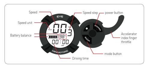
1) Speed step setting Can adjust with button.
