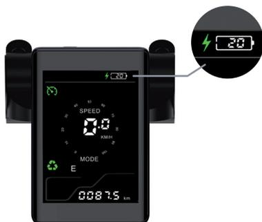
The picto means you have reached the low power protection amount and the electric scooter will lock in ECO mode to save the battery.
